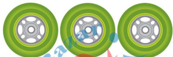
Flat inline skate setup with no rocker
